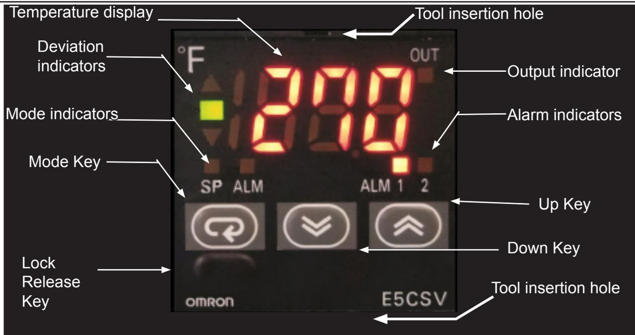
**Omron Model E5CSV Temperature Controller**
