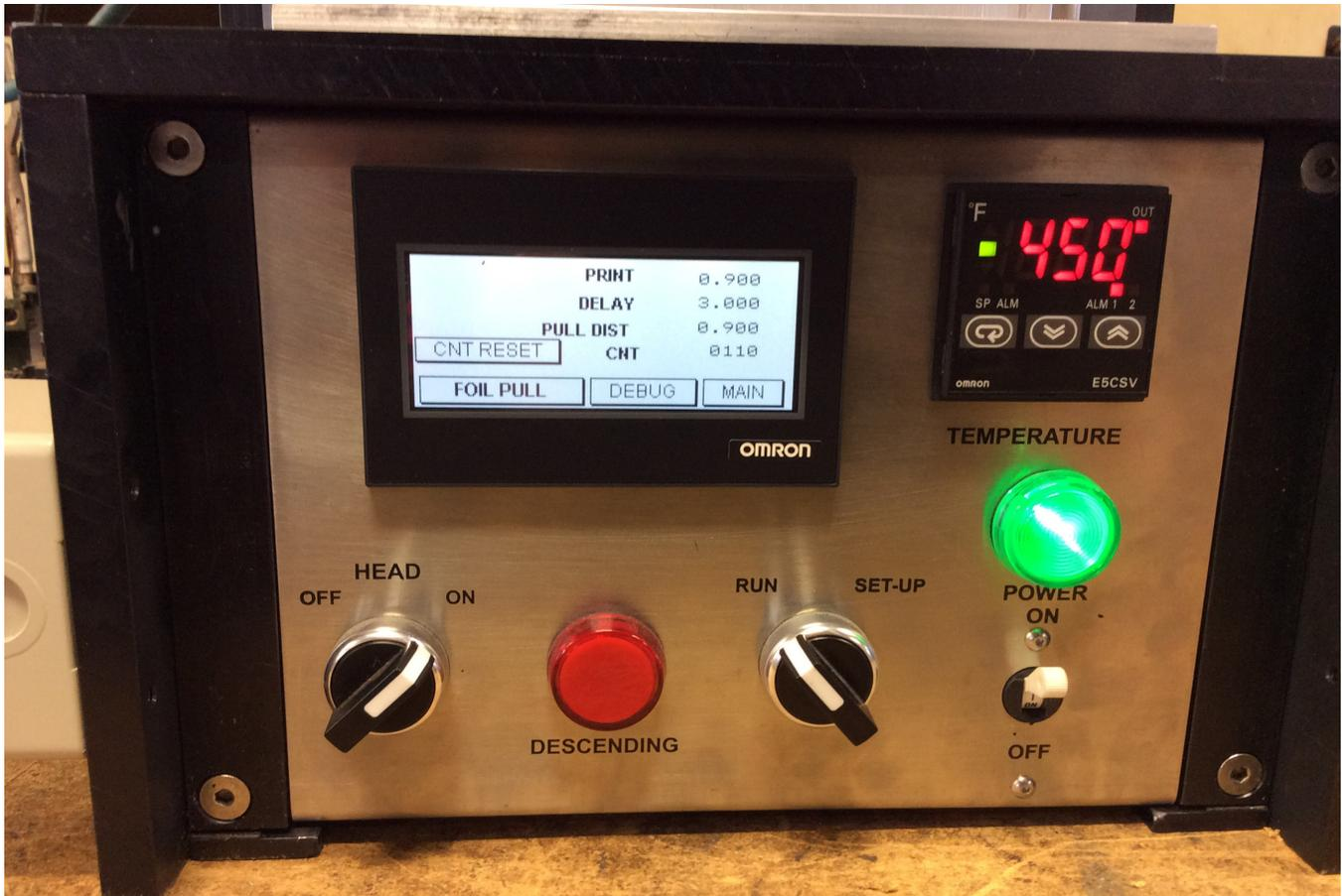
Standard AFM Control Box with an Omron PLC, touchscreen and temperature controller
