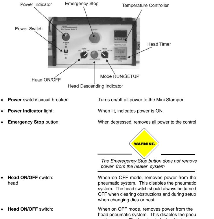
Change the print time by pressing the DIGIT button labeled 4, 3, 2, or 1. Pressing this button will cause the small number to go up one each time. After reaching "9" the digit will go to "0". When you have reached the time setting you want to press RESET. The large number displayed on the timer screen will change to the same as the small number below it.
