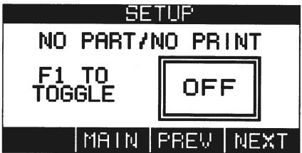
Pressing F1 will toggle from OFF to ON. When set to ON the system will use the part sensor to determine if a part is present. If the part is present the system will print that part (tag). When set to OFF the system will print at every station no matter if a part is there or not.
