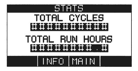
This screen displays the total number of cycles run on this machine in a non-resettable count display.
