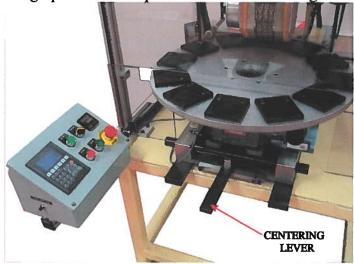
For proper operation of the rotary dial hot stamp press, the foil has to be threaded behind the stripper bar as shown in the following picture.
