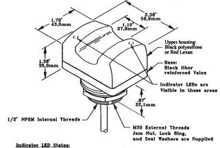
Indicator LED States: LED 1 turns ON when the unit is powered up LED 2 follows the action of the output
