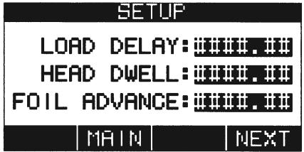
TIMER SETTINGS - This controller is equipped with a number of addressable, internal timers. To set them, press "SET", a cursor will highlight on the first timer. Use the arrow keys to highlight the timer you want to change. Key in the number (don't forget the decimal point) and press enter. That value is stored in memory.
