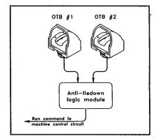
"A two-hand trip shall have the individual operator's hand controls protected against unintentional operation and have the individual operator's hand controls arranged by design and construction and/or separation to require the use of both hands to trip the press and use a control arrangement requiring concurrent operation of the individual operator's hand controls."
