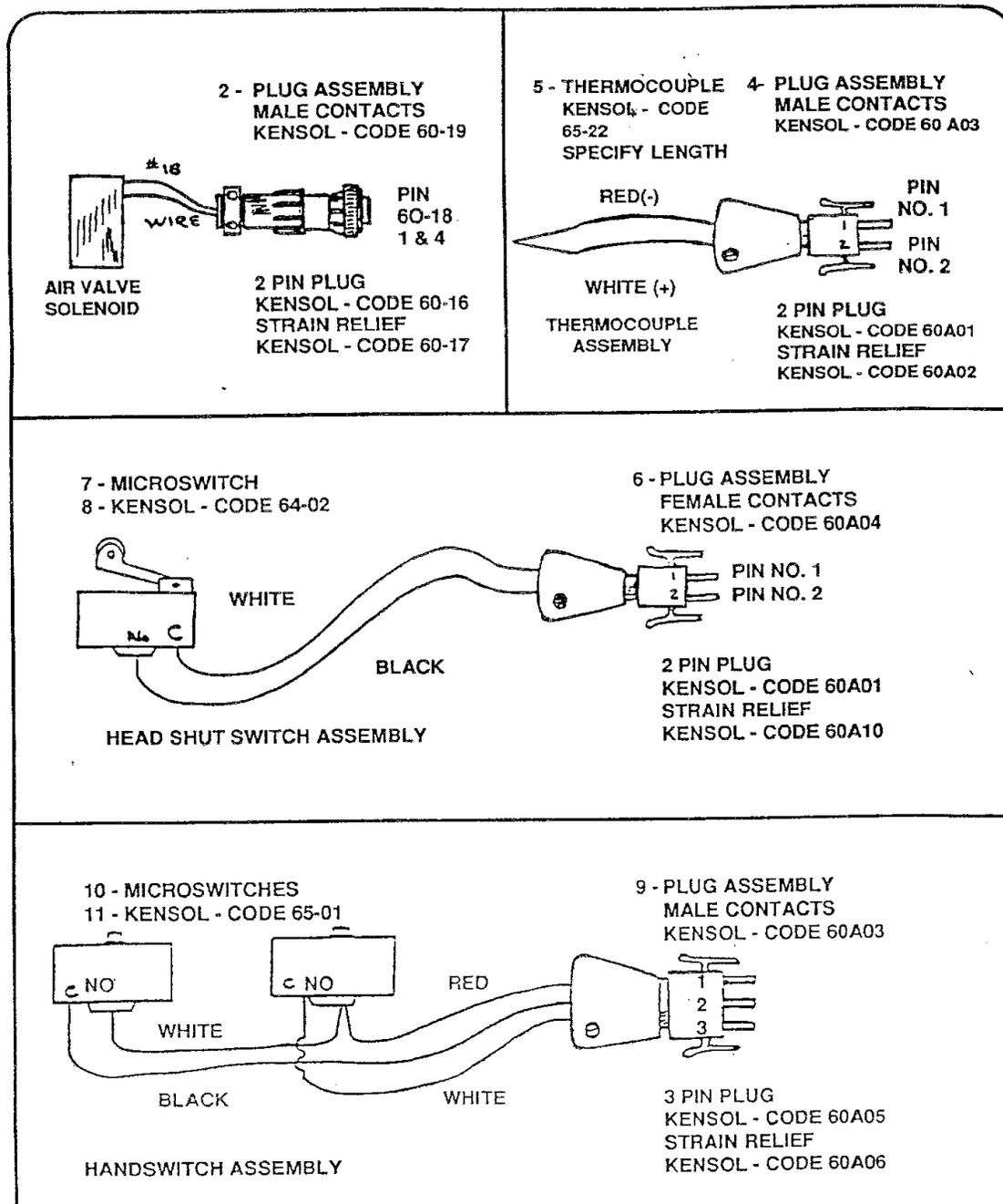
MICROPROCESSOR PLUG WIRING DIAGRAM
