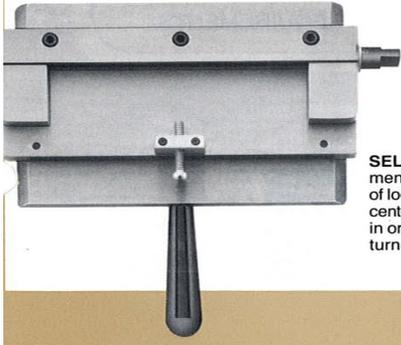
**SELF-CENTERING PALLET** - Recommended for quick change of several lines of loose type or slugs. Pallet automatically centers the lock up because the jaws travel in or out equally when removable crank is turned.
