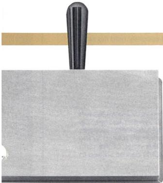
**HOT PLATE CHASE** - 3/4" thick ground steel (or aluminum) plate mounted onto a dove tail plate with a handle. This chase is recommended for mounting flat dies. Dies are mounted using screws, glue or die bonding film. Some customers drill and tap the plate with a hole pattern. The die maker uses a template of this pattern to drill clearance holes that match up with the mounting holes in the chase.
