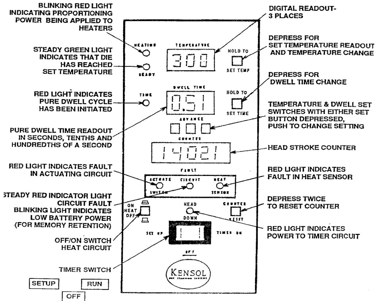
The Microprocessor Switch MUST be left in the "OFF" (Mid Position) when Disconnecting or Connecting the Electricity or Removing Plug
