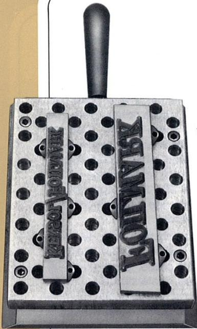
**HONEYCOMB CHASE** - Used to hold thin, inexpensive zinc or magnesium dies. Steel block contains a pattern of special type stepped holes which accept special grippers. The key provided forces the gripping edge of the clip against the edge of the die. If the die is slightly out of alignment, the clips can be shifted to align properly.
