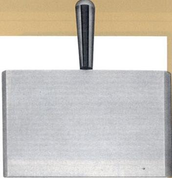
**HEAD SLIDE** - 3/8" thick dove tail plate which is recommended for customers who use type high dies (.918 inches). Plate is normally drilled and countersunk with a clearance hole for screws that mate with drilled and tapped holes in the die.
