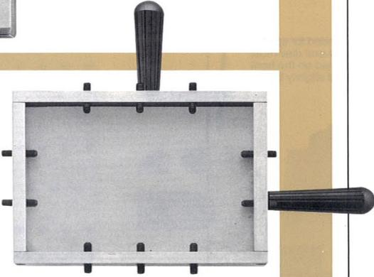
**FOUR WALL LOCK UP CHASE** - Recommended for large lock-ups of type high dies, slugs and loose type. Spacers are required to separate individual pieces of type where required, and metal or wood strips are used to separate lines. The complete lock-up is secured by tightening the set screws found in the side walls.
