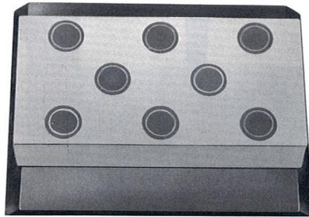
**MAGNETIC CHASE** - One inch thick ground steel block mounted onto a dove tail. Block contains magnetic inserts which will securely hold flat steel dies. Non ferrous dies (silicone rubber, magnesium, copper, brass) could be used if they are first mounted onto a steel plate.
