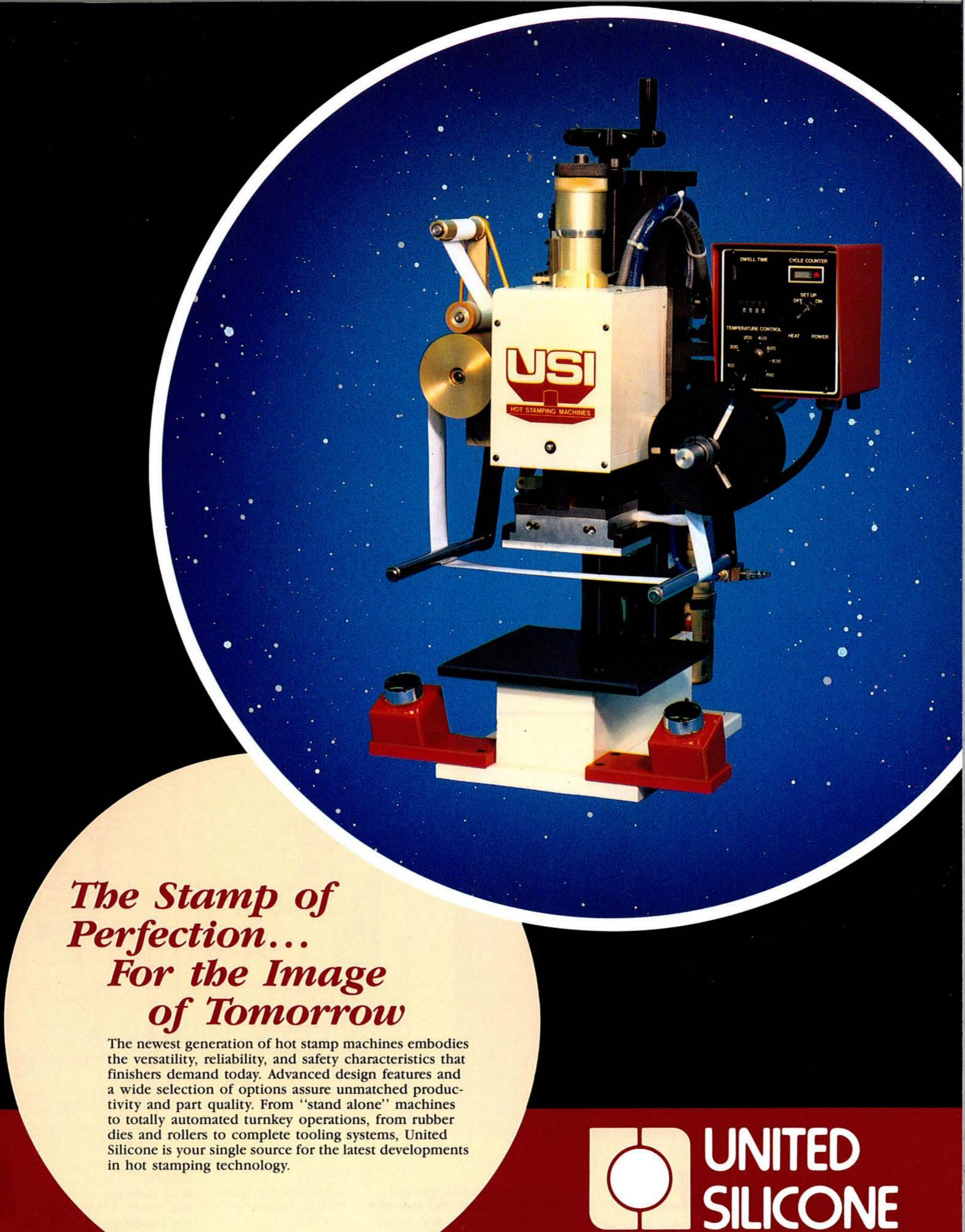
The vertical, pneumatic model US-5 is a solid, yet economical performer. An oversize cylinder rod offers optimum head stability and accuracy. Quick change die mounting, instant spent foil removal, and easy-access control panel enhance operator convenience and improve cycle time.
